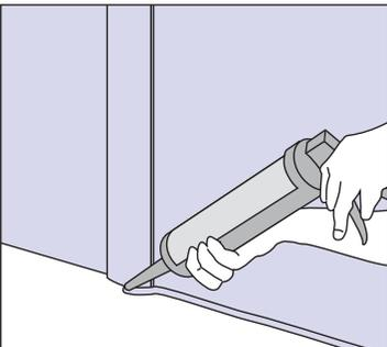
**11** Continue this process to fix panels around each wall and seal gaps at the base of each panel using silicone sealant.
