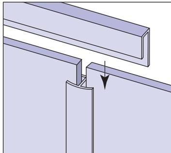
**12** Upper and lower edges may also be finished using end caps. Should this joiner be used, ensure all lengths of vertical sheet joiner finish 11mm short of edges. A bath mould is recommended for the lower edge of panels butting against a bath rim.
