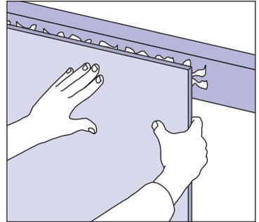
**6** Rub the back of each panel with coarse sandpaper in the areas that will make contact with the adhesive. Work with one sheet at a time, applying adhesive and installing. Position the panel carefully and press firmly to make contact with adhesive. Remove the panel until the adhesive becomes touch dry (approximately 5 to 10 minutes) and follow the adhesive manufacturer's instructions.
