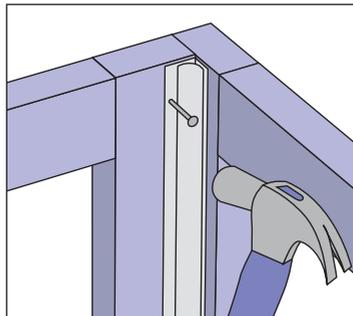
**4** Begin in one corner by nailing or stapling an internal corner joiner to the timber frame.
