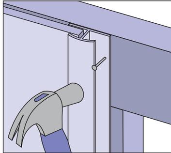
**10** Allow for a 3mm expansion gap on each side of the next joiner and nail or staple the joiner to the frame.
