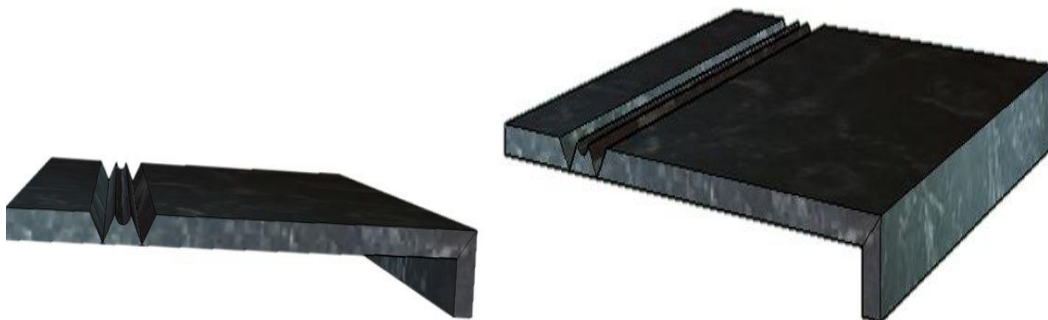
Figure 21. V-Groove edge before gluing and folding
