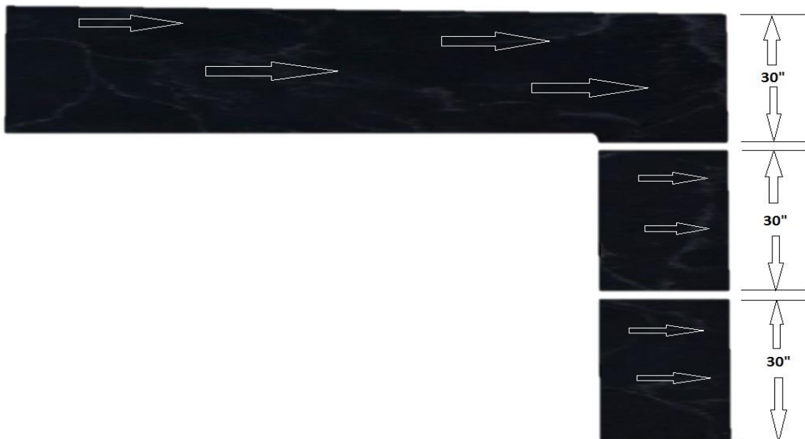
Figure 12. Meganite Movement Series pieces seamed with veining running in same direction, offset inside corner.
